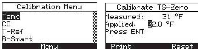
“Measured” is the current temperature reading. “Applied” is a known temperature that will be applied for calibration purposes.
