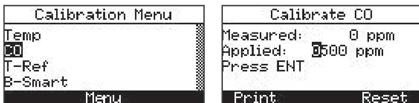
“Measured” is the current CO reading, while “Applied” is a known CO level that will be applied for calibration purposes.
