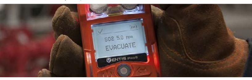
Gas detectors are lifesaving instruments that must be worn in your breathing zone to be effective. OSHA defines the breathing zone as "a hemisphere forward of the shoulders within a radius of approximately six to nine inches," so a collar, lapel, or outside breast pocket is usually a good option. This location also keeps the instrument visible so you can see alerts if your hearing is impaired while working in a high-noise environment.
