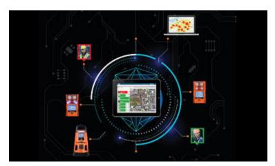
It's no longer sufficient for employees to carry personal gas monitors at all times. New technologies connect entire teams of workers, sharing alarms between devices and alerting everyone to dangerous gas levels. When time is critical and communication is key, instant alarm sharing is a literal life saver.
